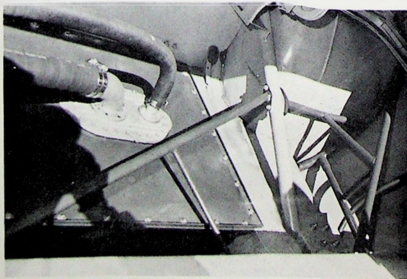
SUPER-CLEAN--These detail engineering photos of Richard Petty's STP-Plymouth show the extra care in engineering which makes the Petty-produced machines consistent winners in NASCAR racing. Upper left, detail of roll-cage in rear section of cab, with differential cooling unit in background. Upper right, left front suspension detail, showing massive brake, and cooling duct. Lower left, space-frame tubing in trunk with resilient couplings to prevent troublesome fender damage. Lower right, sanitary cockpit with fully-instrumented dashboard and auxiliary instrument panel.
