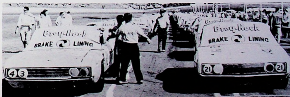
CARS ARE LINED UP before the start of the National 500 at Charlotte, N. C., on October 12. Each windshield was covered with an aluminized asbestos cover to reduce intense heat buildup in the cockpit from the sun's rays. Covers can also be used to smother sudden pit stop fires, or as protective barrier against steaming hot radiator water. Grey-Rock has made a limited supply of these windshield covers for NASCAR drivers.
