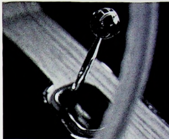
The Hurst shifter climbing out of an extra-cost console covered with walnut wood grain styling.
