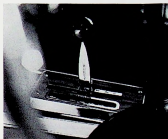
Extra-cost Turbo Hydra-Matic with Hurst quadrant. Right slot is for manual stick shift control.
