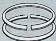
Two-piece interlocking ring provides Gapless Seal
