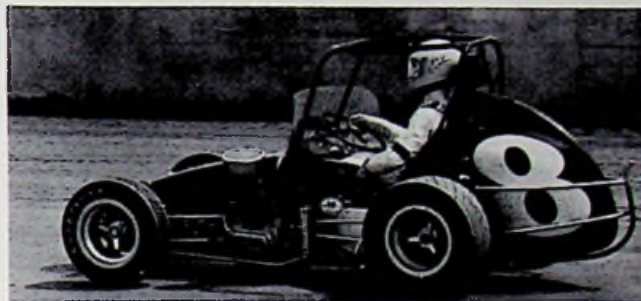
Roll bars were superseded by full roll cages and they became mandatory in USAC in 1971. This is Rich Vogler utilizing Volkswagen power in 1979. USAC News photo by Ralph Tippy.
